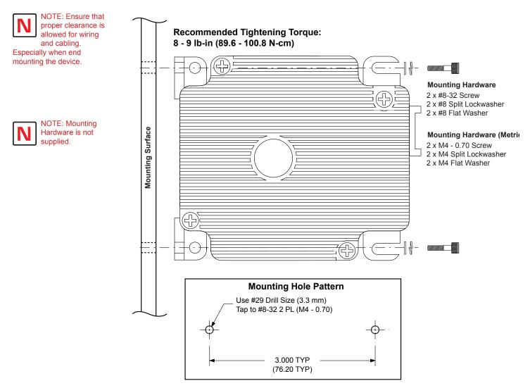
Figure 2.1.2: End Mounting the MForce PowerDrive
